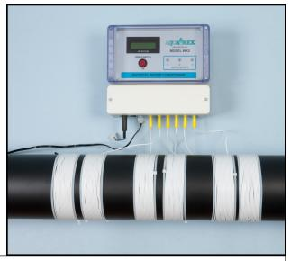
of each pair must be wound in opposite directions from a central point. When facing the pipe, one aerial should start by passing behind the pipe and the other should pass in front of the pipe. Secure each end of the aerial with a cable tie. Leave a gap of at least 1" between each aerial. Repeat the process with the other pairs of aerials.
