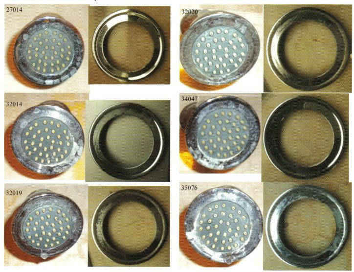
On 29th March 2011 the hotel occupancy was very high and we were only able to inspect the shower head in 32020. Pictures were taken of the chrome ring in the condition it was taken off the head. A picture was taken again after wiping with a soft towel and removing a little scale with the thumb nail. The results showed that the ring cleaned up completely as it had done on January 26th, two months earlier.
